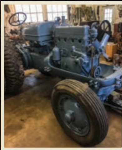
The I-9's 4-cylinder gasoline engine had 4\frac{13}{32} \times 5\frac{1}{2} -inch bore and stroke and ran at 1,500 rpm. IH also built the ID-9 with a diesel engine.
