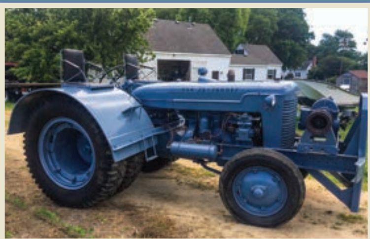
Seats mounted on the fenders were used by the ground crew members who had to hitch and unhitch trailers and connect air brakes.
