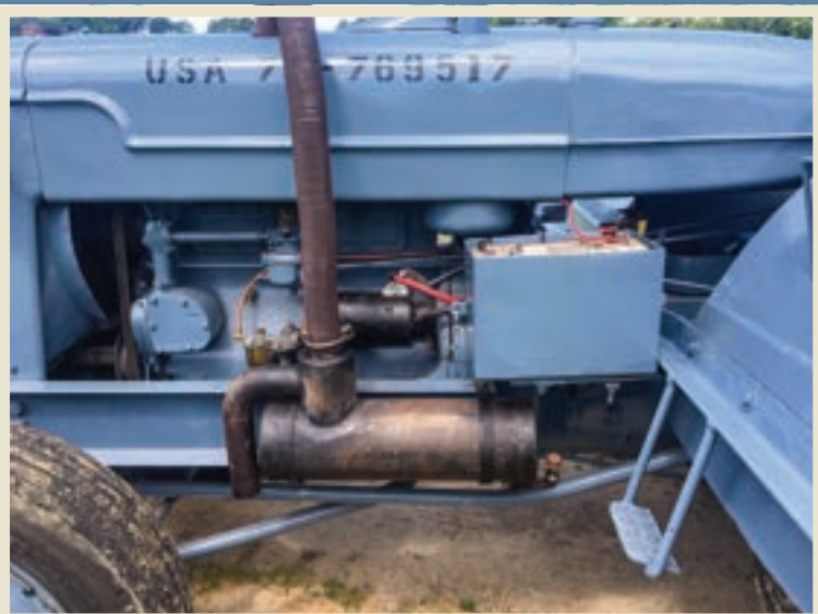
The I-9 Special has a water-bath exhaust spark arrestor system to make the tractor safe when hauling trailers filled with explosives.
