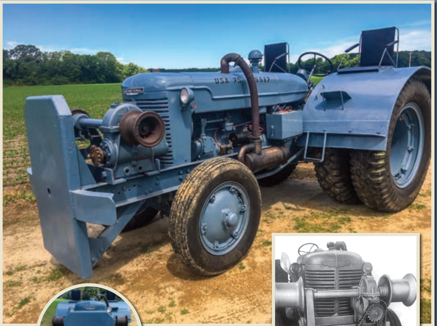
The Gar Wood front-mounted double capstan winch was driven by a shaft from the tractor's crankshaft.
