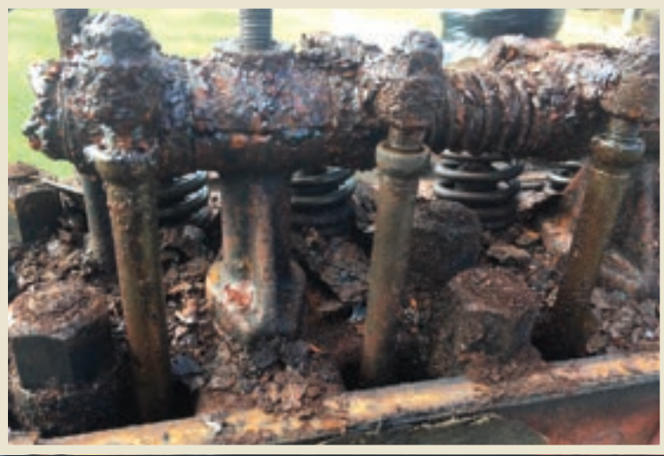
These will not simply “buff out!” Luckily, the I-9 Standard held a wealth of spare parts, including engine valve components.
