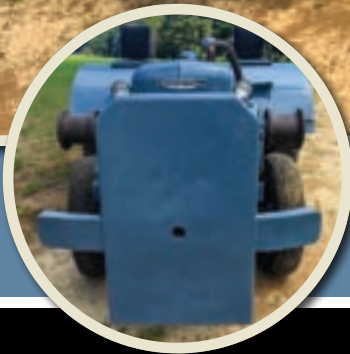
The Gar Wood front-mounted double capstan winch was driven by a shaft from the tractor's crankshaft.
