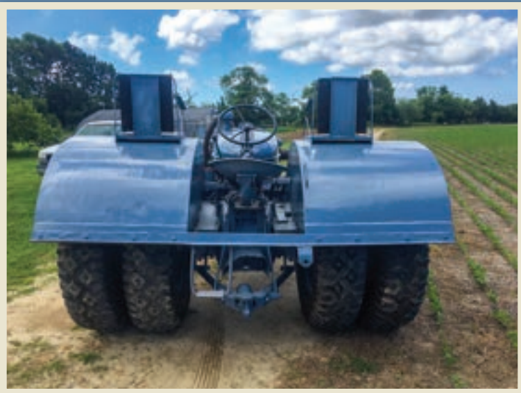
Seats mounted on the fenders were used by the ground crew members who had to hitch and unhitch trailers and connect air brakes.
