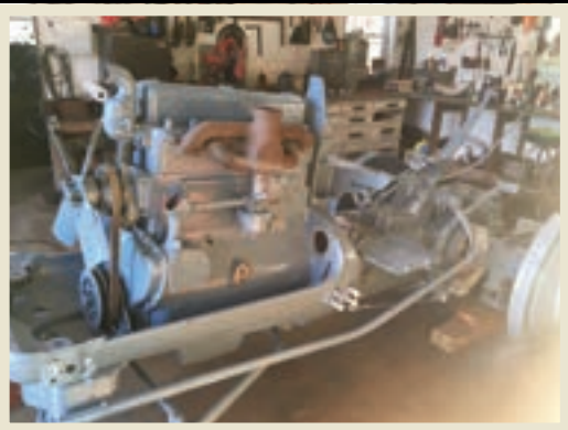
The I-9's 4-cylinder gasoline engine had 4\frac{13}{32} \times 5\frac{1}{2} -inch bore and stroke and ran at 1,500 rpm. IH also built the ID-9 with a diesel engine.
