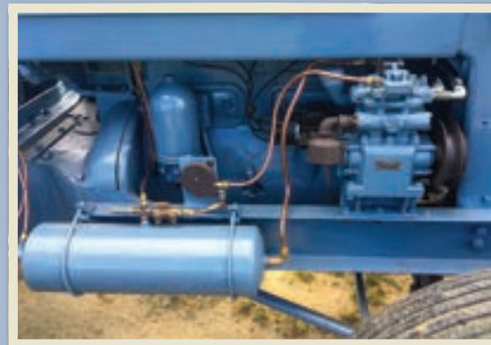
A Bendix-Westinghouse air compressor produced air for the air brakes on attached trailers.
