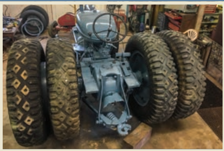
The heavy-duty hitch testified that the I-9 Special was a genuine pulling tractor.
