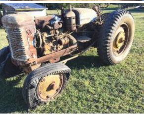
exhaust system that extends across the hood and down into a water bath spark arrestor. Excellent details were shown in the manual. He says the exhaust was built that way, so the tractor was safe for hauling fuel and trailers filled with explosives.
